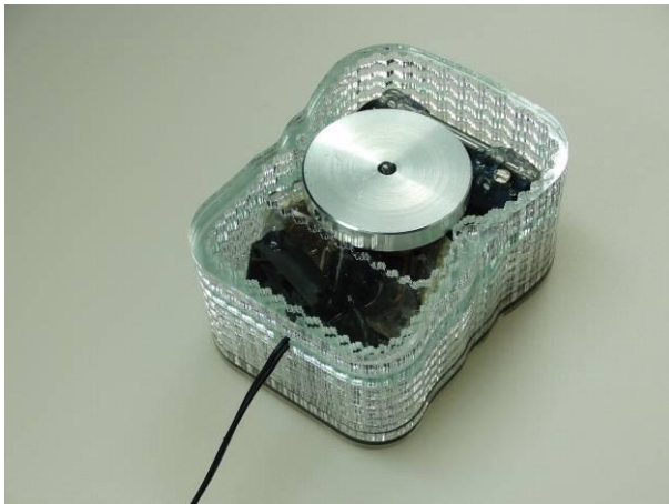
Figure 6. The accelerator is composed of three units: an acceleration unit, a gyroscopic unit and an impact-force unit.
